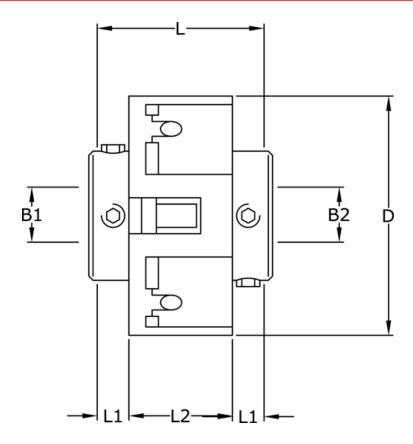
$\begin{array}{lll} B1 & = 6 \\ B2 & = 6 \\ D & = 34 \\ L & = 25.2 \\ L1 & = 8.1 \\ L2 & = 8.9 \\ Screw = M4 \end{array}$
